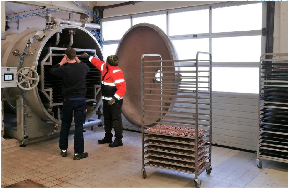
1000 EKS-R with 90m 2 tray area, 1.000kg capacity
